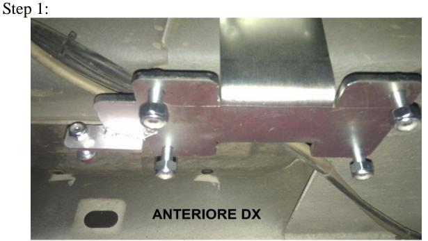
Put the adapter on the frame approximately under the cab seats, most rear possible, if necessary remove any sealing material for a perferct adherence, use a bottle jack to stop the bracket in the correct position and make the 8mm side hole then fix with the bolt.
