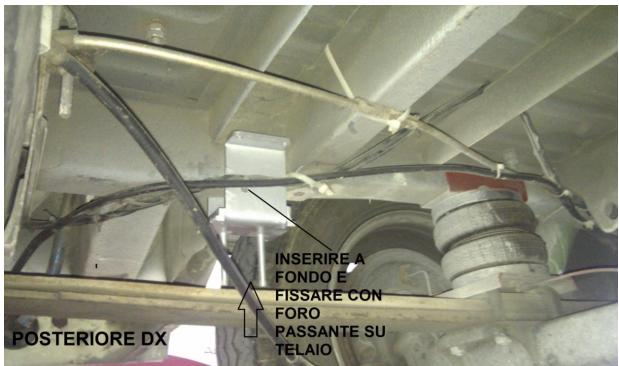
The rear adapter must be placed before the rear axle
