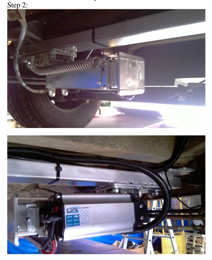
BOTH REAR JACKS WITH ENGINE TO THE REAR OF THE VEHICLE AND INSIDE ROTATION
