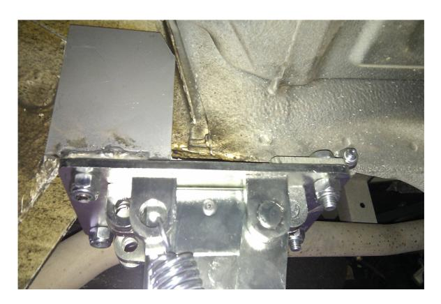
JACK WITH MOTOR TO THE OUTSIDE OF THE VEHICLE AND ROTATION REAR
