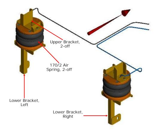
In addition to the parts illustrated above, the kit comprises of...
