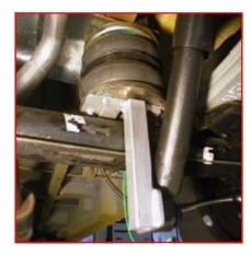
Figure 3. Placement of the Air Spring
