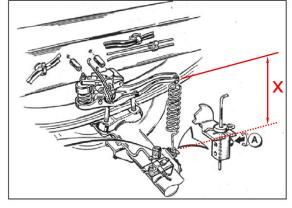
between the upper and lower mounting points, as originally measured as a preliminary step (see Page 8), then re-tighten bolt (A)
