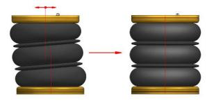
**CAUTION!** - Before fully tightening the bolts that secure the air spring to the upper and lower brackets, set the vehicle at ride height (spring height approximately 18..22 cm) and ensure that the springs are correctly aligned.
